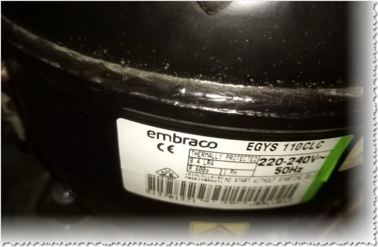
Mbsm.pro, Compressor, Embraco, EGYS110CLC, 1/3 hp, lbp, r600a, 263 w, 1.1a
