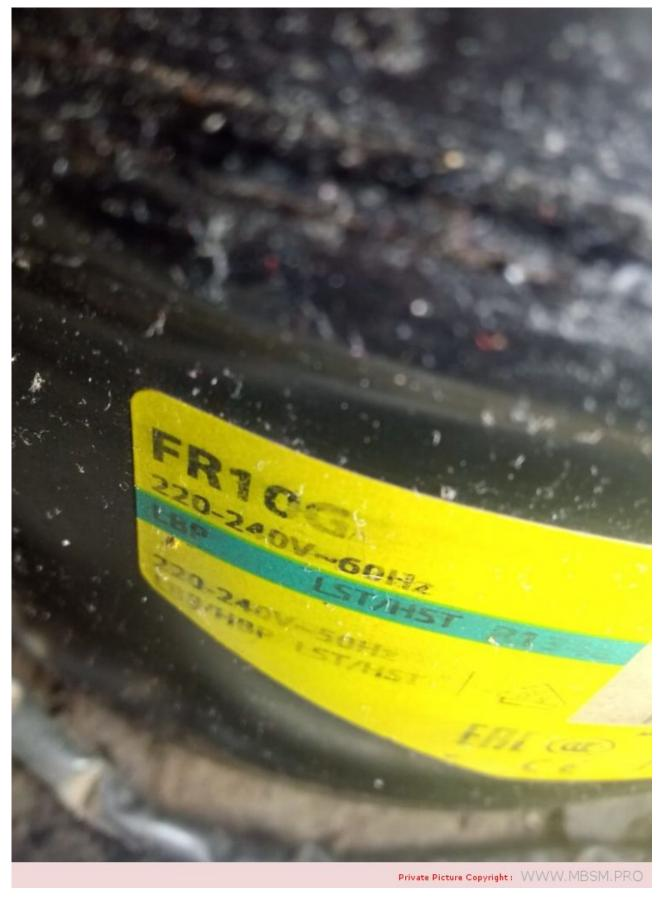
Mbsm.pro, COMPRESSOR, SECOP, FR10G, R134a, 1/4 Hp++, 1/3 Hp-, HMBP, 103G6880-HST, DANFOSS, CSIR, 730 BTU, 9.05 cc
