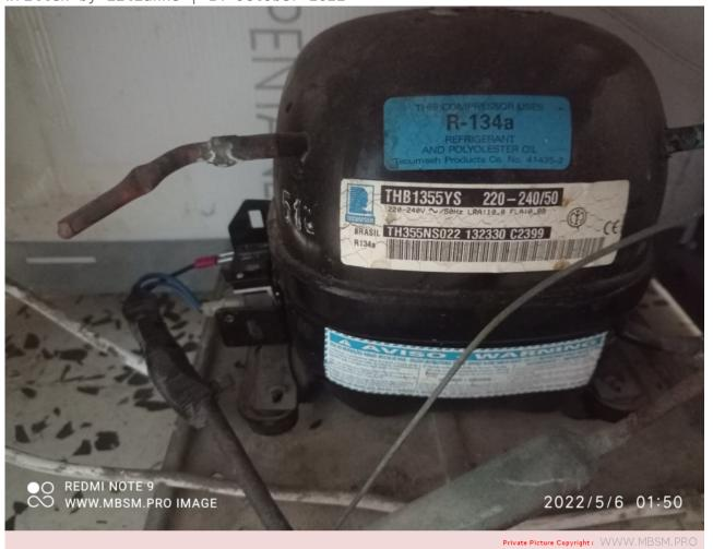
Mbsm.pro, Freeser, Ariston, ECH240s1, 240 L, Compressor, TECUMSEH BRASIL, THb1355y, 1/5 hp, LBP, R134A, 100g, replaced by, egm70af, gl70aa, capillarie 0.026, 1.2 m, Alert -10
