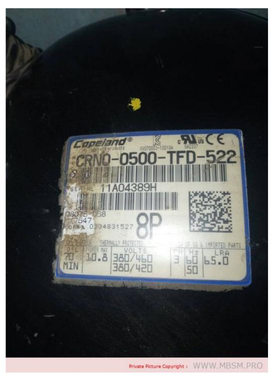
Mbsm.pro, Copeland, Reciprocating, Hermetic, Compressors, CRNQ-0500-TFD, 5 hp, R22, HCFC, R-22, 50 Hz, 3 — Phase,  $380/420\ V$ , CR QR Series
