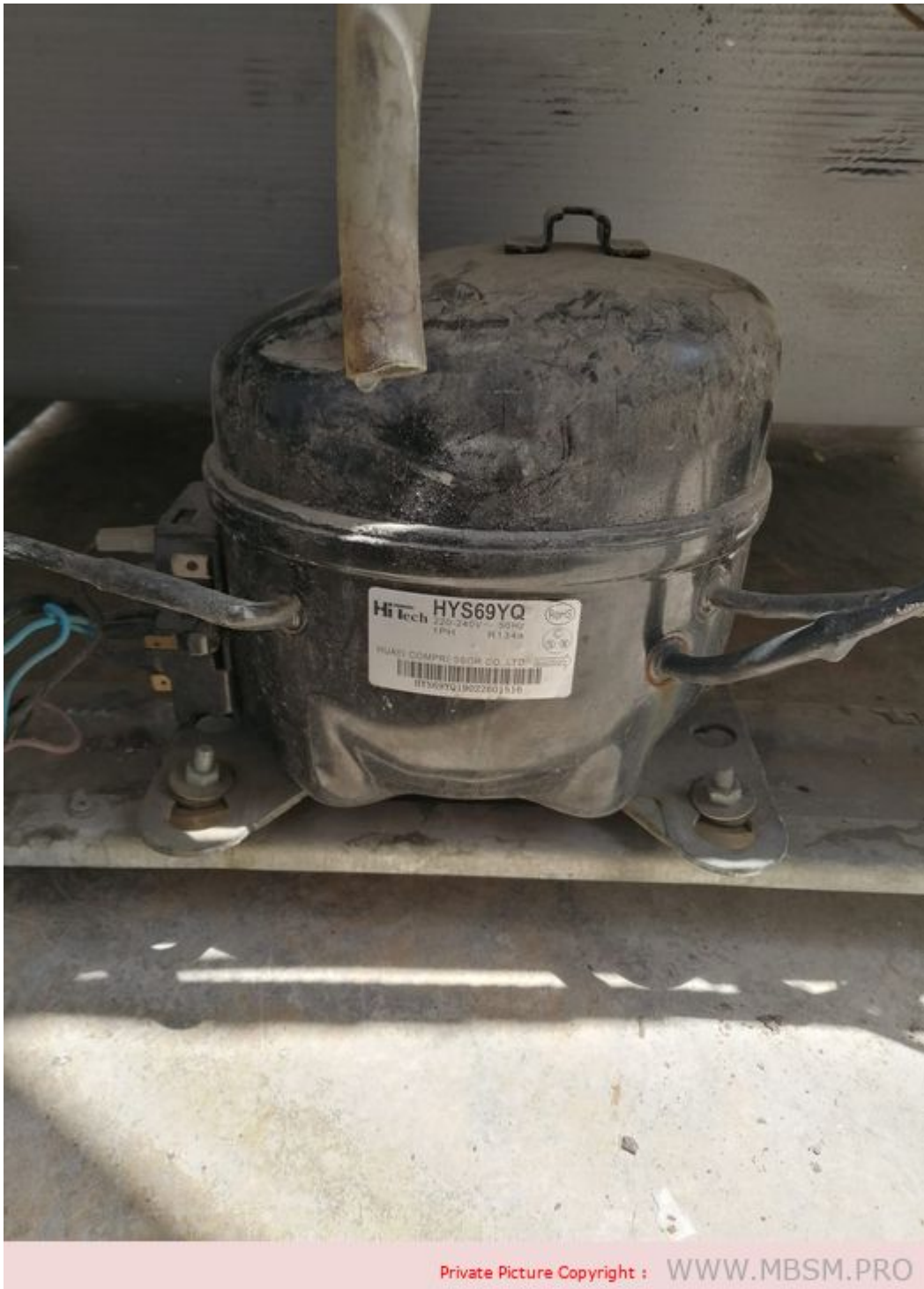
Mbsm.pro, Compressor, hys69yq, 1/4 hp, 1bp, HiTech, r134a
