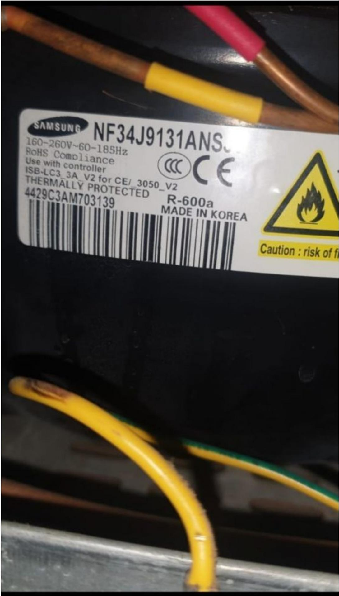
Mbsm.pro, Compressor, NF34J9131AN, 1/3 hp, inverter compressor, form 94 w to 283 w, 240V~50Hz, 220V~60Hz, BLDC, R600a, LBP, Samsung
