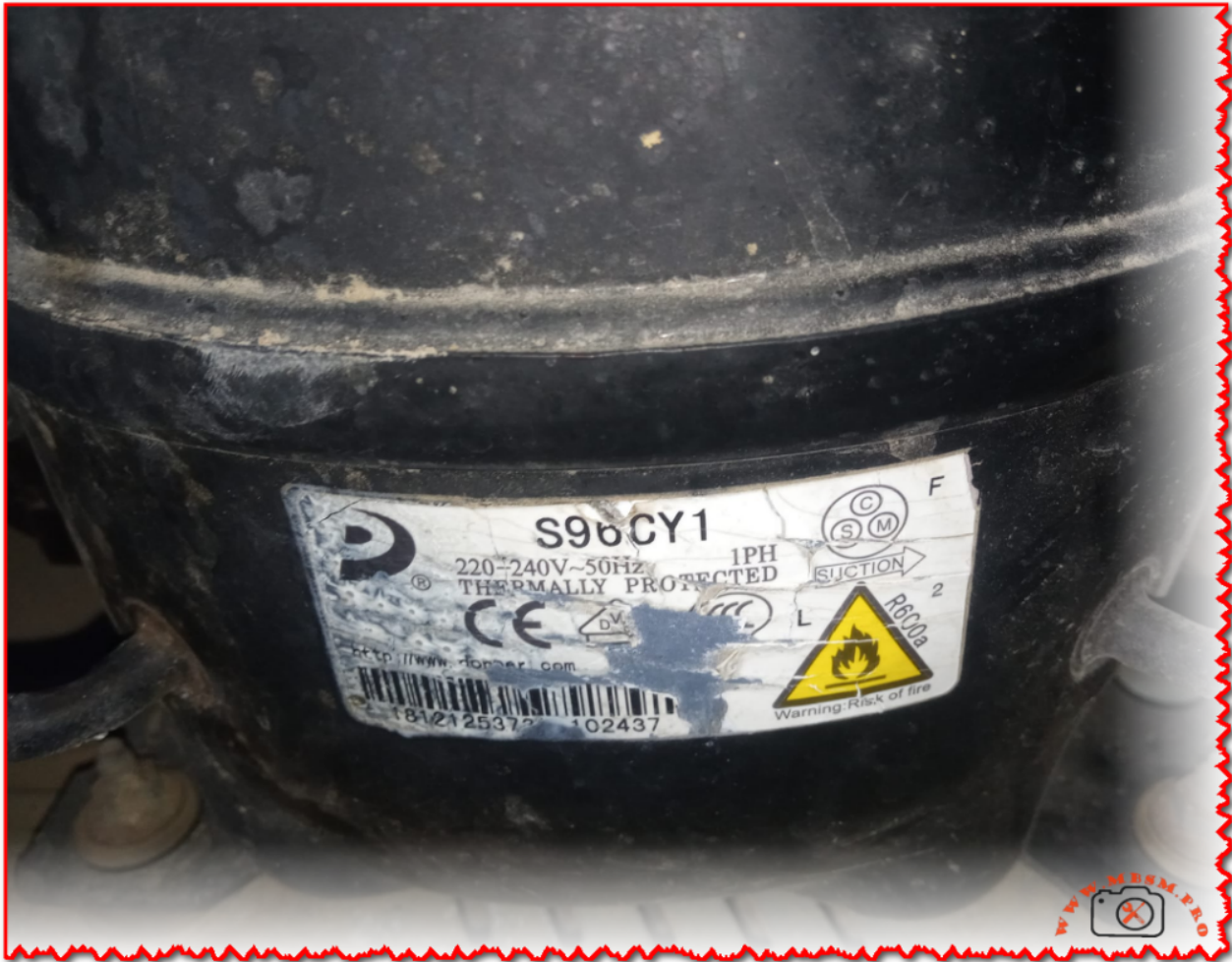
Mbsm.pro, DONPER, Refrigeration, Compressor, S96CY1, H170CY1, R600a (56 g), LBP, 240V 50HZ, 1/5 HP, 155W, CHEST FREEZER, Nikai, NCF340N5, Nikai 340L Chest Freezer
