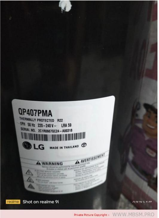
Compressor, LG, QP407PMA, 2.5 hp, r22, 24045 btu, 7048 w
