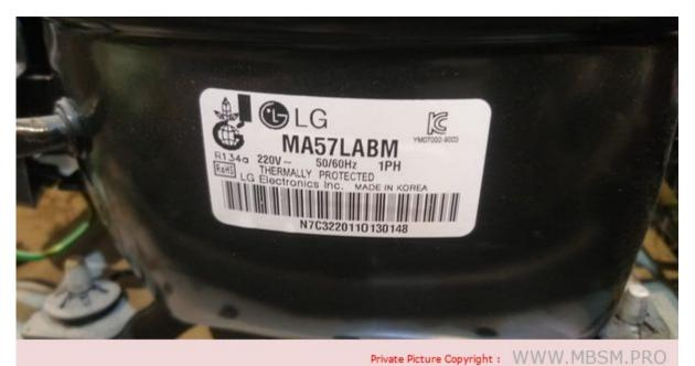
Mbsm.pro, Compressor, MA57LABM, 1/5 hp, 160 w, Lbp, Refrigerator, LG, GR-B562YC
