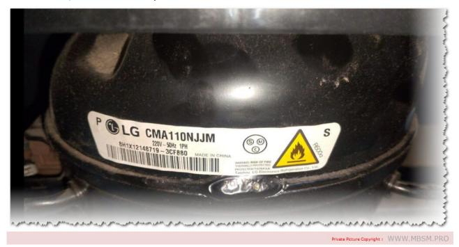
The LG CMA110NJJM compressor is a classic model that operates on a single phase with a voltage of 220V and a frequency of 50Hz. It boasts a fixed speed and is powered by a 1/4 HP motor. This compressor is perfect for applications requiring a steady and reliable performance.
