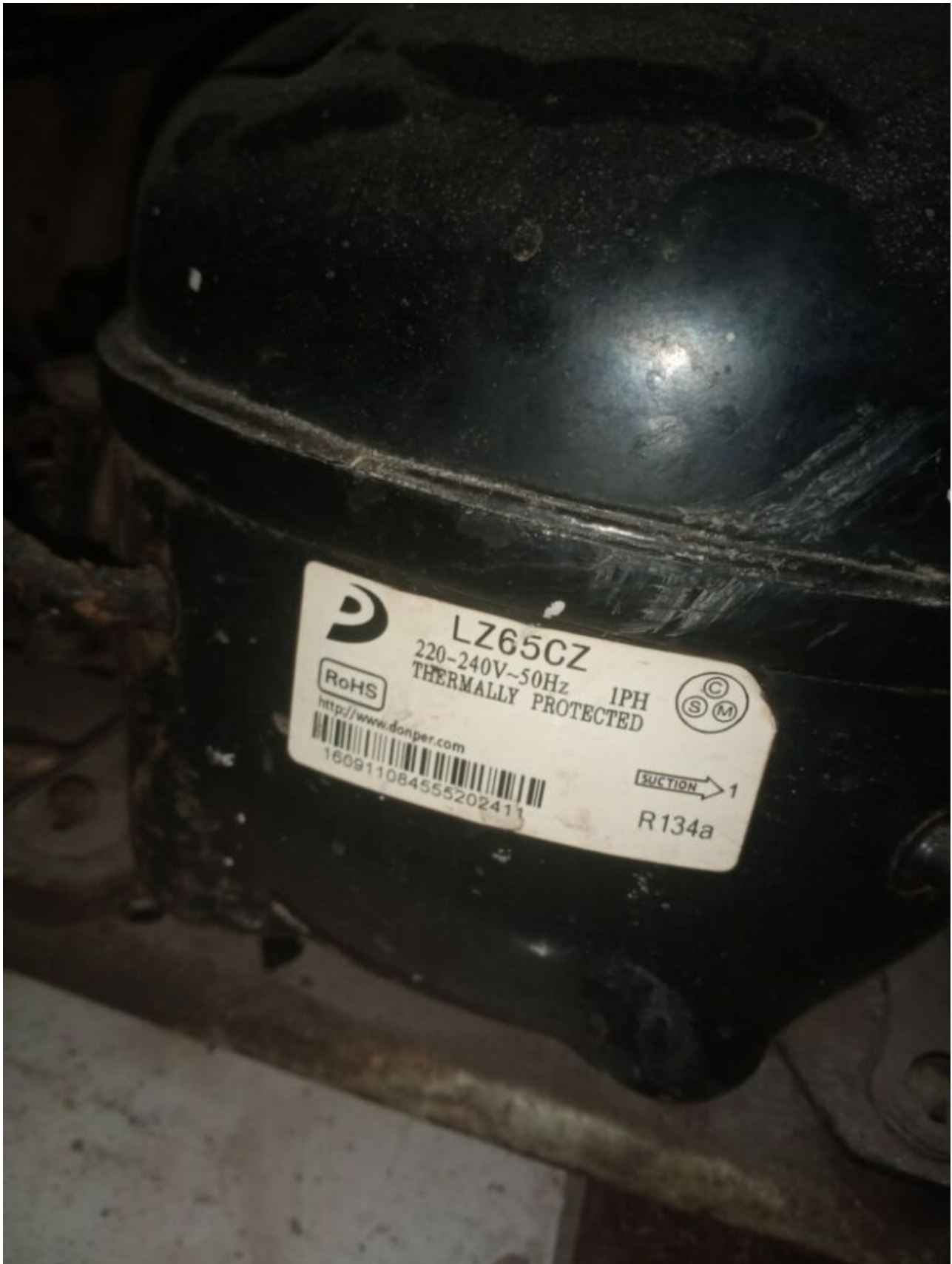
Mbsm.pro, Compressor, Lz65CZ, 1/5 hp, r134a
