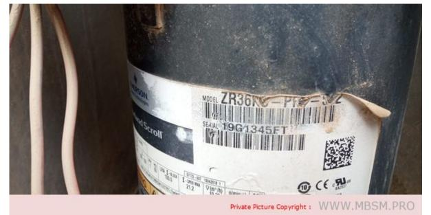
Mbsm.pro, 30000 BTU, Copeland, Scroll, Compressor, ZR36KC-PFJ-522, 3 Ton, r22,
