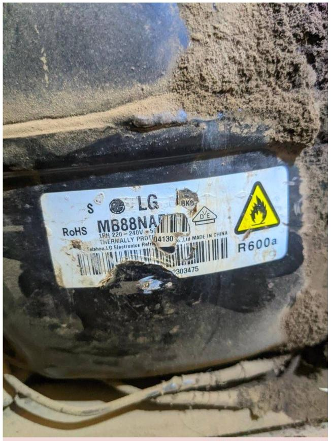
Private Picture Copyright: WWW.MBSM.PRO Mbsm.pro, Compressor, Lg, Lbp, MB88NA, 151 w, 1/5 hp, r600a, 1ph-220v-50hz
