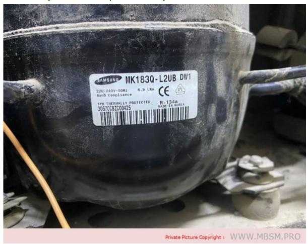
Mbsm.pro, NFD, 620 L, Full No Frost, refrigerator , Teka, compressor, MK1830-L2UB, 1/3 hp, lbp
