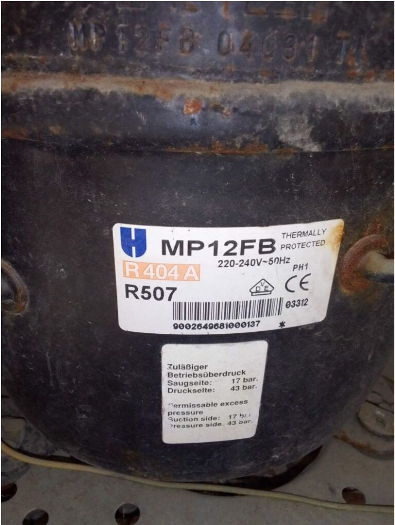
Mbsm.pro, Compressor, Cubigel, MP12FB, MPT12LA, SC12CL, 3/8 hp, R404A / R507, lbp
