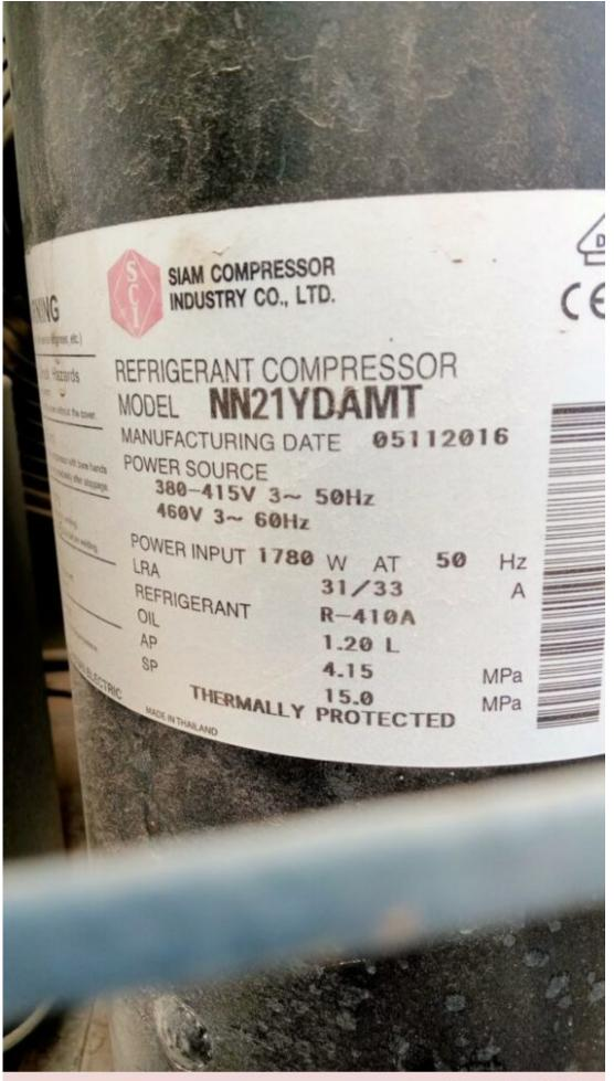
Mbsm.pro, R-410A, Fixed Speed, Rotary, Compressor, Mitsubishi, NN21YDAMT, 1.74 hp, 18000 btu, 3 Ph, 380 v
