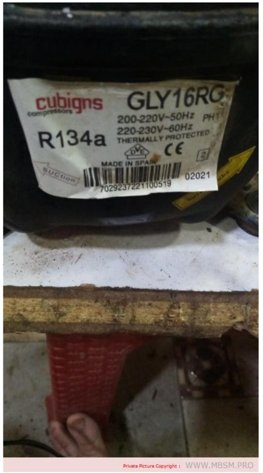
Commercial refrigerator, compressors, GLY16RG, 3/8 hp++, R134a, HMBP, 1492W,
