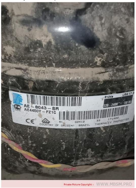
Mbsm.pro, compressor, AE 4450 Z, AE4450Z, AE4450-Z-FZ, AE4450Y-AA1A, AE4450Z-FZ1A, HMBP, r134a , 1/3 hp ++,
