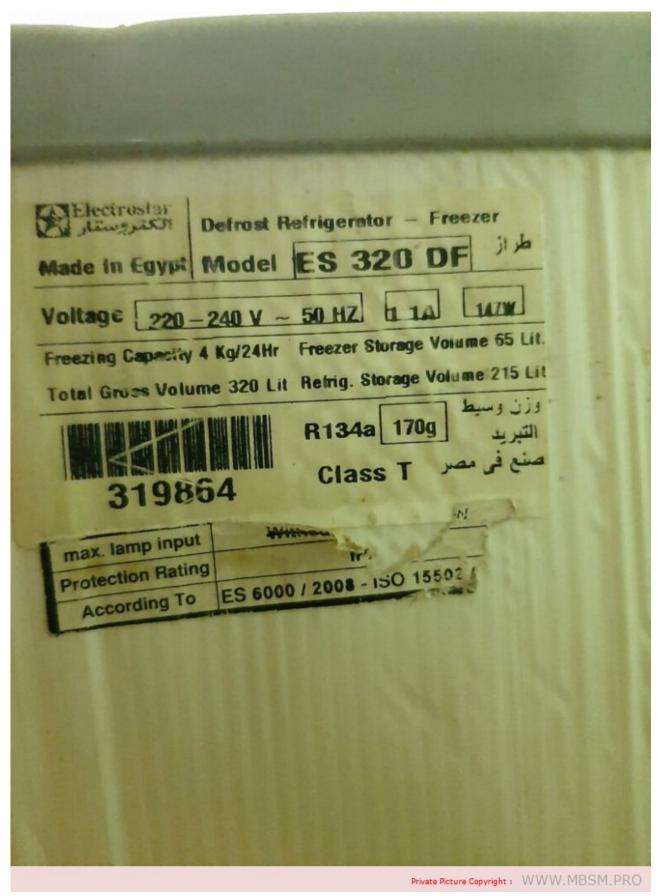
Defrost refrigerator, ES320DF, Electrstar, 320 L, compressor, 1/5 hp, 147 w, r134a, 170 g, 220 v / 50 hz, lbp
