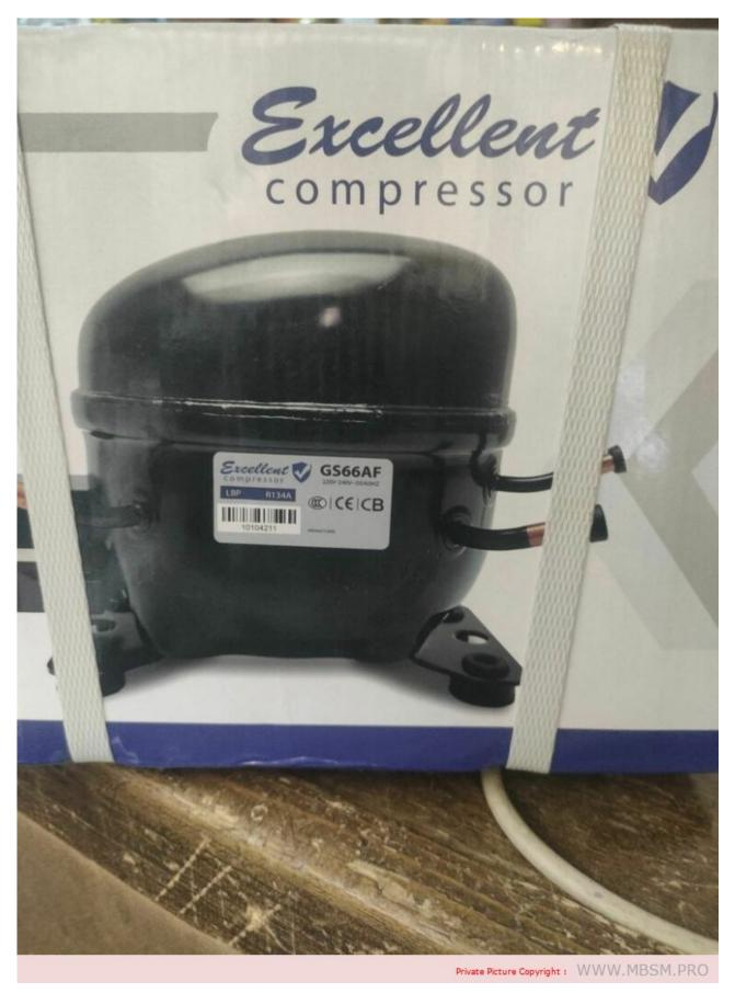
Excellent, Compressor, GS66AF, 1/6 hp, LBP, r134a, disp 6.6 cm3, 165 w, 1Ph, 220 v/50hz , GS77AF, 1/5 Hp, GS-90TB, 1/3 hp
