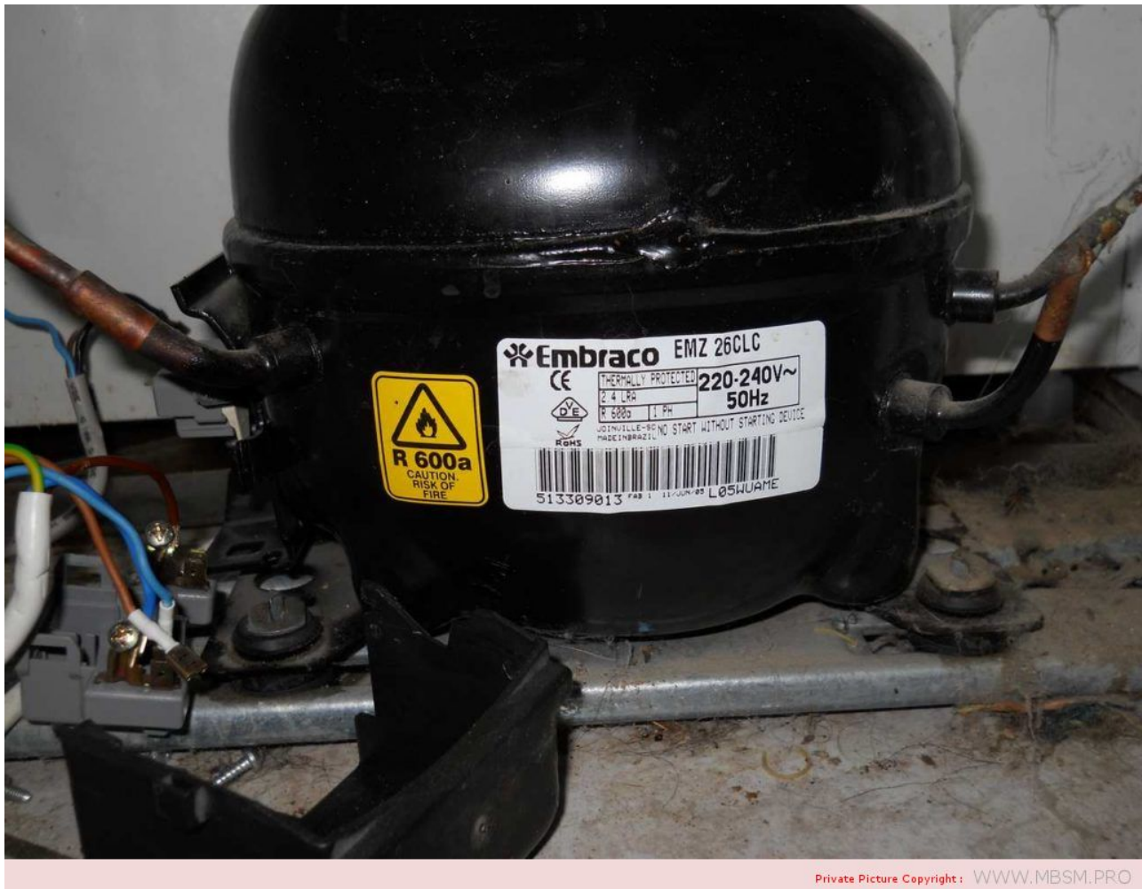
Compressor, Embraco, Aspera, EMY26CLC, LBP, R600a, 220 – 240V/1/50Hz, 1/12 HP, RSIR, LRA 7.8 A, 83 Wat
