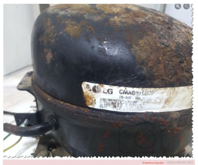
Mbsm.pro, LG, CMA057LHEG, 1/5 hp, R134A, 135 g, Alu Wire, compressor, lbp, 160 w, 1ph, BCD-192, SWAIDY, REFRIGERATOR
