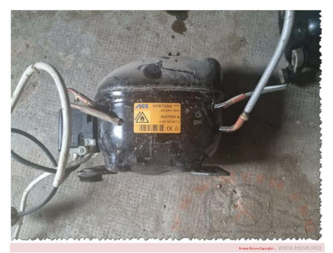
Mbsm.pro, Compressor, HYK12AA, HTK12AA HMK12AA, HYK12AA, REFRIGERATOR, 1/4 hp, lbp, r600a, 197 w
