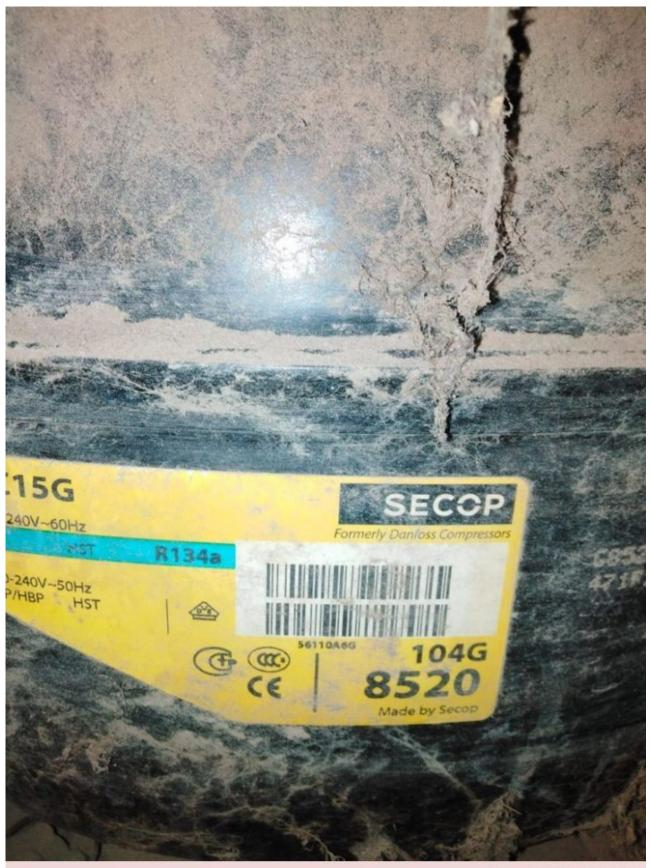
3/8HP Danfoss secop refrigerator compressor SC15G 104G8520 for R134a
