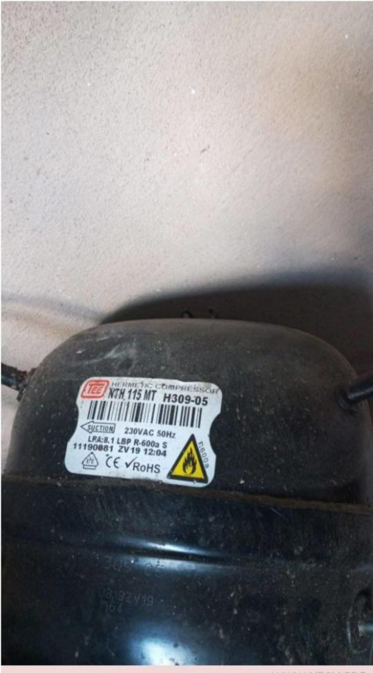
Mbsm.pro, compressor, refrigerator, NTH115MT, Turk Elektrik, 115 Kcal/h, 1/5 hp, TEE compressor, r600a, lbp, BEKO Fridge Freezer Compressor, 220 v
