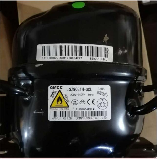
Mbsm.pro, Compressor, cGMCC, refrigerator, SZ90E1H-SCL, 1/4 Hp, R600 A , 220 v 60 Hz
