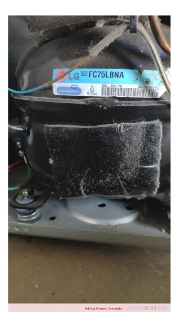
LG, Refrigerator, Compressor, FC75LBNA, TCA35271202, Inverter, AR125VC, R134A, 1/3hp, 0-220V 53HZ
