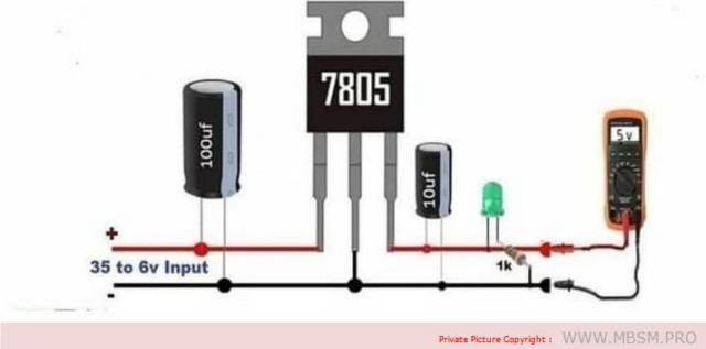
Mbsm.pro, 7805, 12/5Volt, Regulator, Circuit, Diagram
