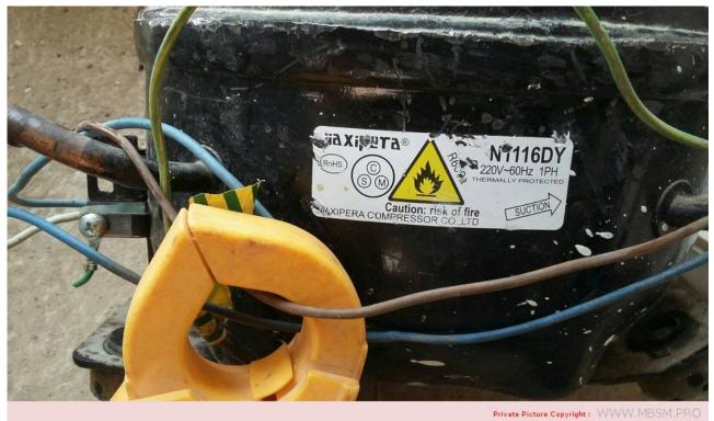
Mbsm.pro, COMPRESOR, N1112dY, 1/6 Hp, N1116dY, 1/5 Hp, LBP, JIAXIPERA, R-600a, 4  $\mu$ F, RSCR, 220-240 $\sim$ /50
