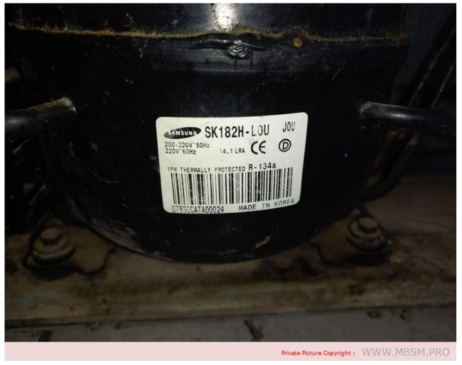
Mbsm.pro, Compressor, SAMSUNG, SK182H-L2U, 1/4 hp++, 1/3 hp -, 236 w, 806 BTu, Rscr, lbp, r134 a
