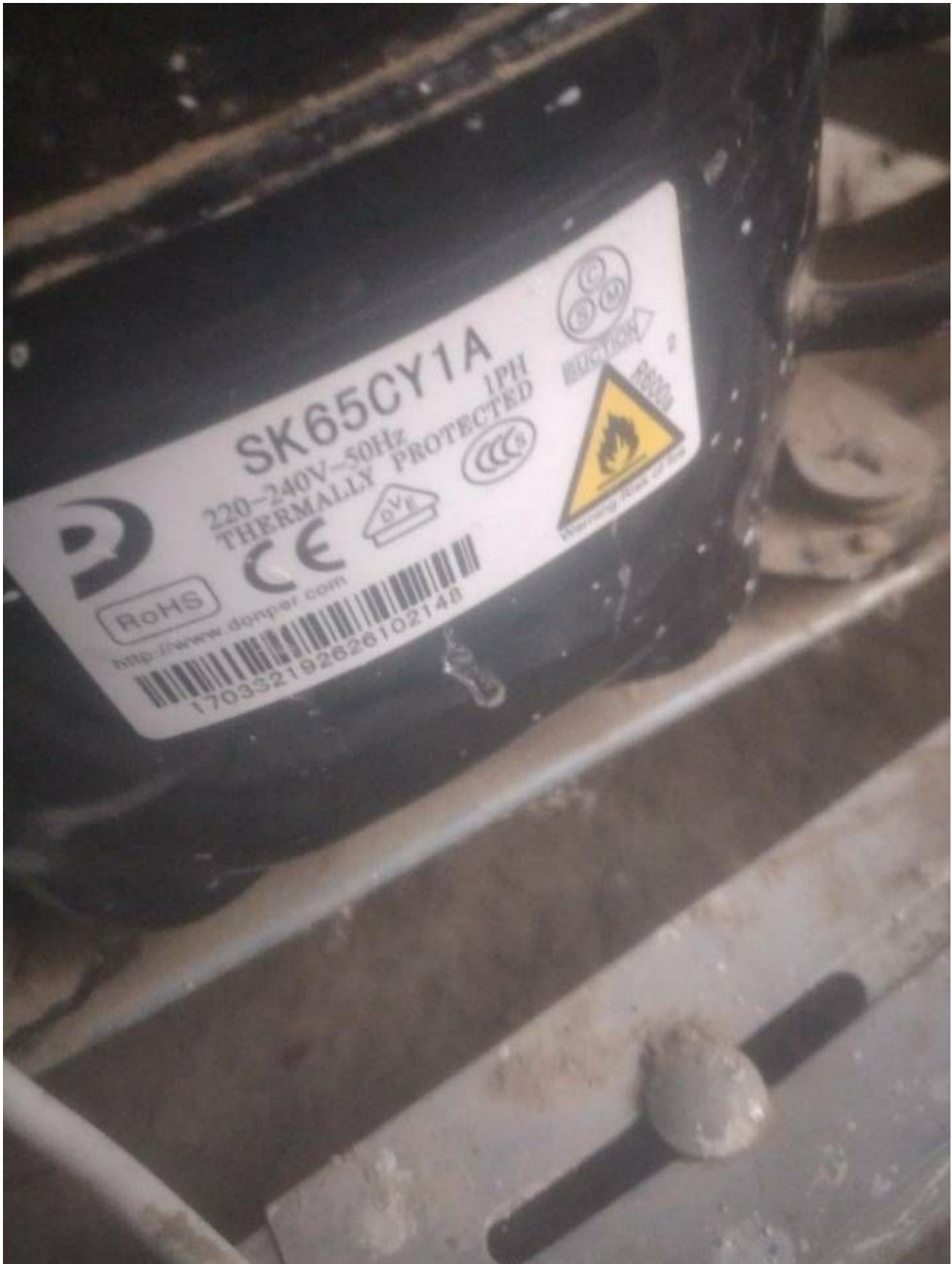
Mbsm.pro, COMPRESOR, Domper, SK65CY, R600A, 1/8 HP
