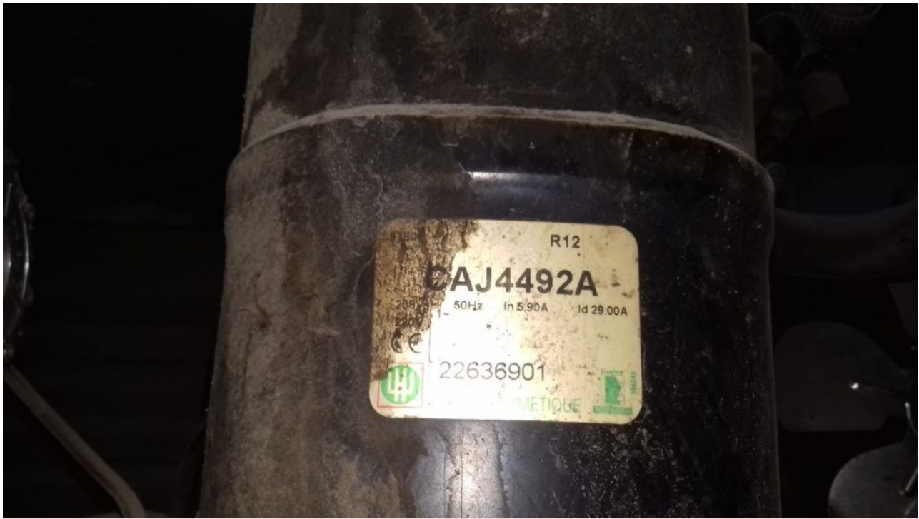
Caj4492A, R12, Tecumseh, Refrigeration, Compressor, 3/4HP, Medium/High Back Pressure
