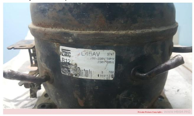
Mbsm.pro, Compressor, Electrolux Group, Zem, Compressor, L45AV, R12, 1/8 hp, HMBP
