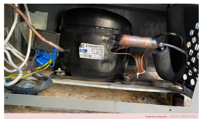
Mbsm.pro, compressor, EGM60AF, zmc, Manufacturing Compressor Misr , 1/6 hp, LBP, RSIR / RSCR
