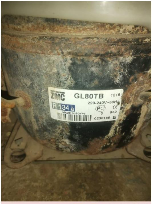
Mbsm.pro, Compresor, ZMC, 1/5 hp++, 1/4 hp-, High-Medium Back Pressure, GL80TB, GL80AA, cooling and freezing
